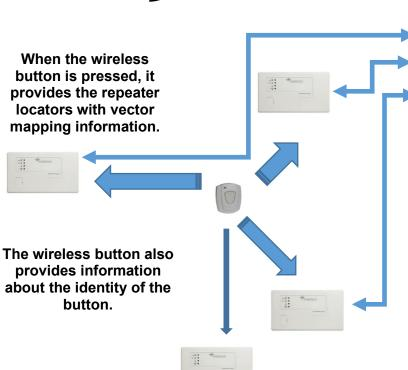
A message detailing the location of the button and its identity is transmitted by radio and, if needed, by email and/or text message.
