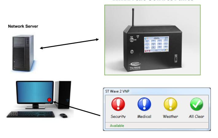
Virtual buttons provide a way to distribute buttons to a large number of desk based personnel within a computer network. Any Windows based computer within the LAN can have up to four customizable virtual buttons installed.
